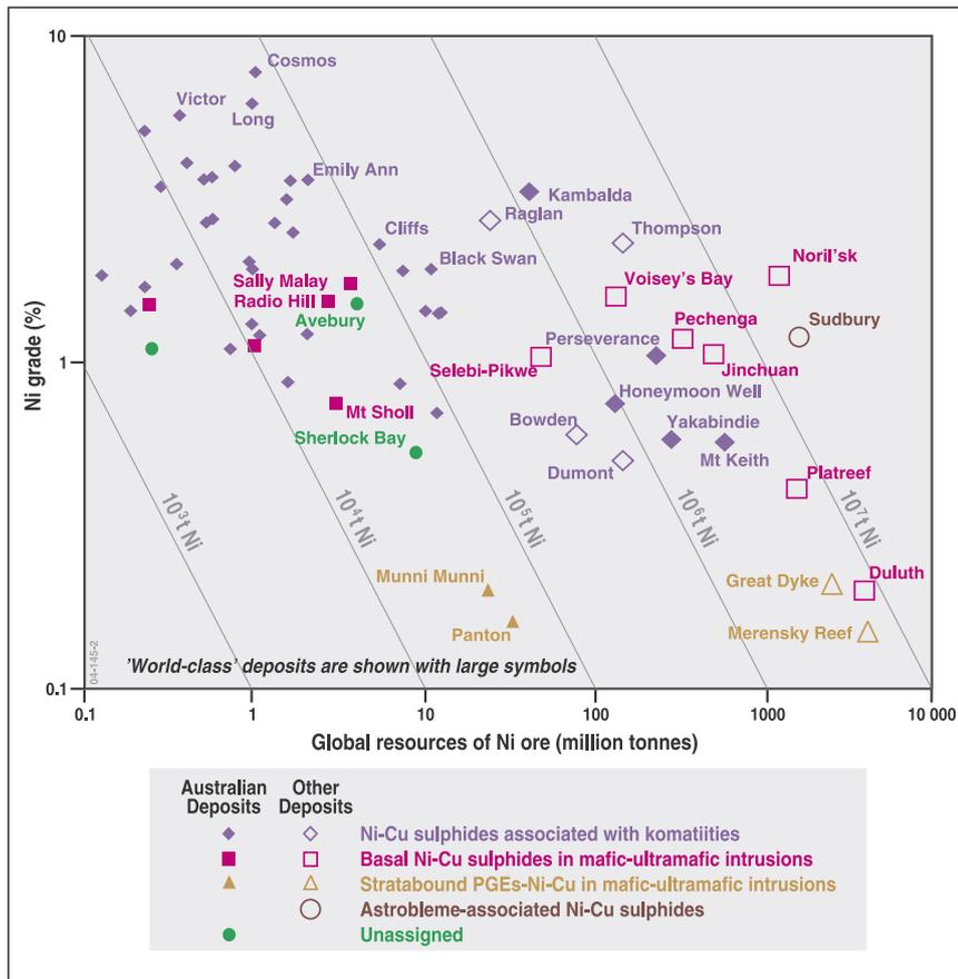
◀ **Figure 2.** Logarithmic plot of nickel grade (wt%) versus global resources of nickel ore (production plus reserves and resources in million tonnes) for the major nickel sulphide deposits of the world. Australian deposits are shown with filled symbols and other deposits with open symbols. The grey diagonal lines show contained Ni metal in tonnes (source of data: OZMIN 2004, Naldrett 2002, Eckstrand 1995).
