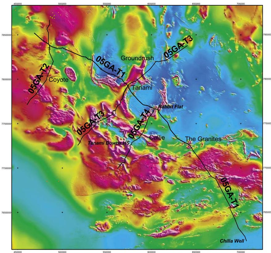
▲ **Figure 1.** Location map of the Tanami region, northern Australia, showing the four Tanami traverses (05GA-T1 through to 05GA-T4). The dotted portion of 05GA-T1 indicates extra kilometres collected due to additional funding and excellent crew performance. A total of approximately 720 line kilometres were recorded. Locations of mineralisation are shown as circles.
