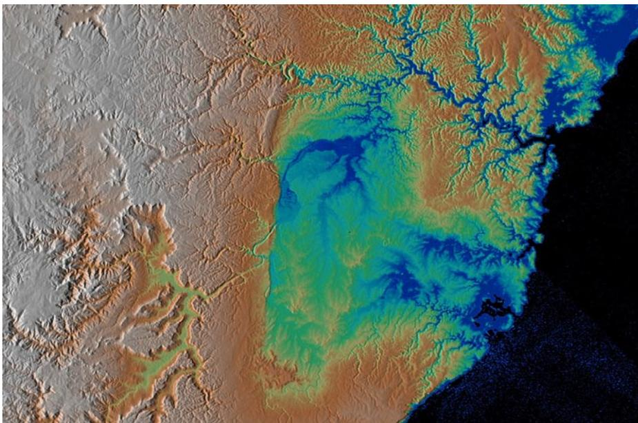
▲ **Figure 1.** SRTM 3-second Digital Elevation Model over the Sydney Basin. The Lapstone Structural Complex is the northerly trending linear feature in the middle of the image. Sydney CBD is in the centre-right.
