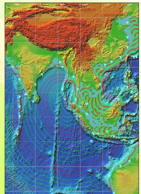
▲ **Figure 3.** Travel-time contours for the Boxing Day tsunami. The source zone is roughly constrained by the tsunami arrival times at the Vishakapatnam and Cocos Islands tide gauges. (the latter is indicated by the magenta inverted triangle southwest of Indonesia). Contours are at 15-minute intervals, and alternate colour every hour. (Figure generated using software provided with the Integrated Tsunami Database for the Pacific, by Slava Gusiakov.)
