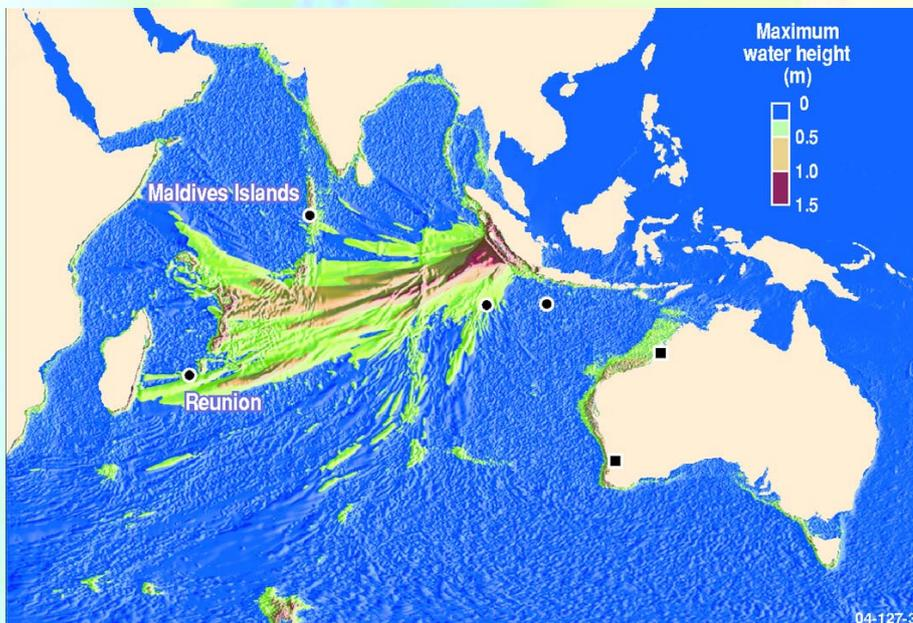
▲ **Figure 2.** Calculated maximum amplitude of the tsunami caused by 1833 Sumatra earthquake. Most tsunami energy was directed into the open Indian Ocean, away from the Bay of Bengal. (Numerical modelling performed by David Burbidge of Geoscience Australia.)
