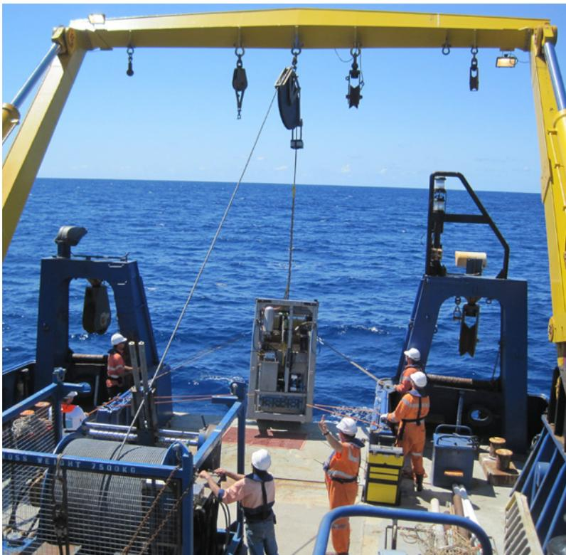
**Figure 1.** The remotely operated vehicle being deployed from the Australian Government's Marine National Facility the RV *Southern Surveyor* during the marine survey searching for evidence of natural hydrocarbon seepage sites in the offshore northern Perth Basin. The RV *Southern Surveyor* is owned and managed by CSIRO.
