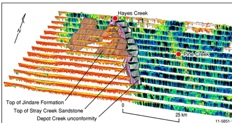
**Figure 2.** Conductivity-depth sections of the Pine Creek area in 3D plus a 3D model of part of the Daly and Birrindudu basins.
