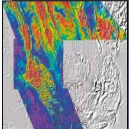
**Figure 2.** An airborne electromagnetics image (colour) draped over an airborne magnetics image (greyscale), central-west New South Wales. The image shows the conductivity modelled for the interval 40–50 metres below the surface. Red colours are more conductive (related to more saline groundwaters); blue colours relate to either resistive bedrock or fresher groundwaters.
