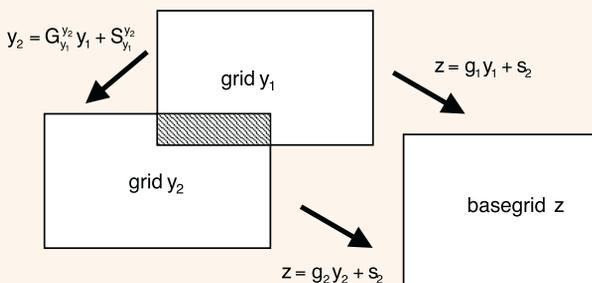
▲ **Figure 2.** The relationship between the relative shift and scale for overlapping grids, and the absolute shift and scale to a base grid. The various terms are defined in the text.
