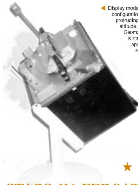
◀ Display model of SUNSAT, which is similar in size and configuration to FedSAT. A magnetometer is mounted on the protruding rod, which is used to provide approximate attitude determination based on the International Geomagnetic Reference Field model. When the satellite is stabilised, a star camera (the box with the hooded aperture) provides accurate attitude information. A sensitive magnetometer is located on the tip of a 2.5-meter boom shown here in its pre-launch position.
