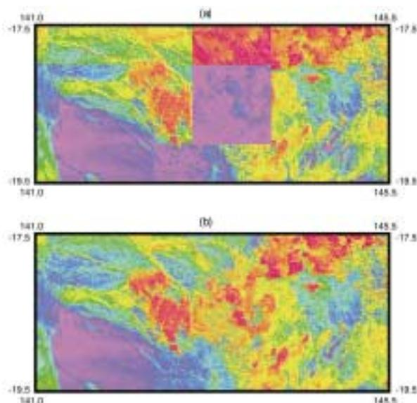
▲ **Figure 3.** Automatic grid levelling of airborne gamma-ray spectrometric data from North Queensland, Australia: (a) composite grid of total count before levelling, and (b) after levelling.
