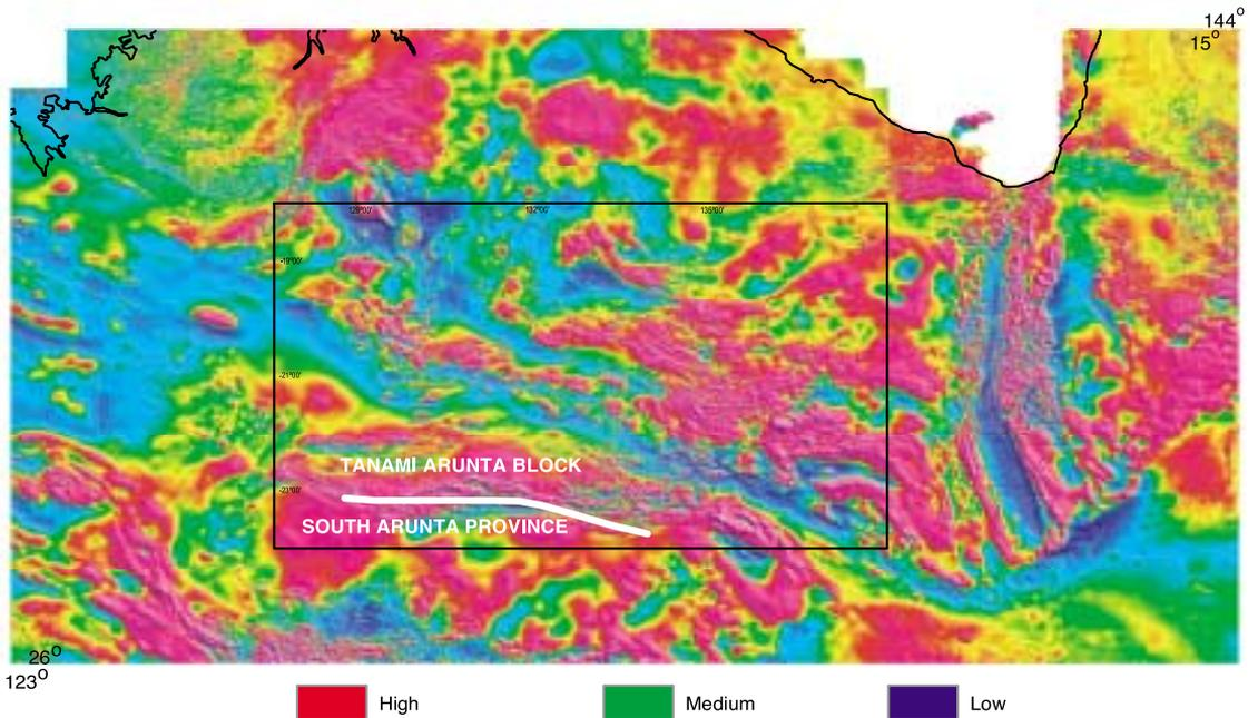
▲ **Figure 6.** Aeromagnetics of the Tanami, Arunta and Tennant Creek regions. Note the broadly east–west-trending, linear magnetic low.
