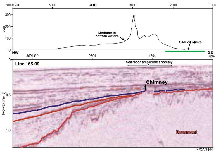
▲ **Figure 4.** Sediments are pinched out, a chimney forms, and hydrocarbons leak into the ocean.
