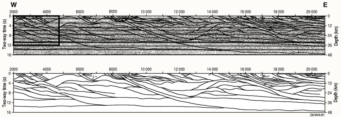
▲ **Figure 2.** Northern Yilgarn interpreted seismic reflection section (top) and interpretation only (bottom)
