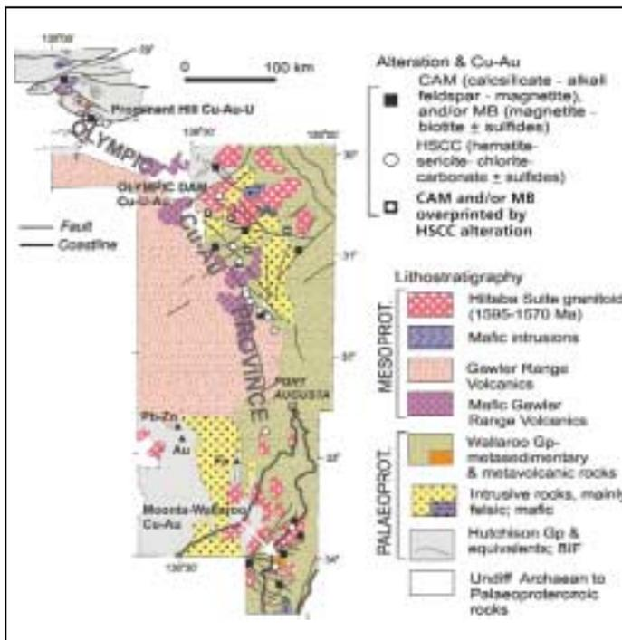
▲ **Figure 3.** Interpreted basement geology (pre-Neoproterozoic) of the Olympic Cu-Au province, and distribution of hydrothermal alteration types in drill holes
