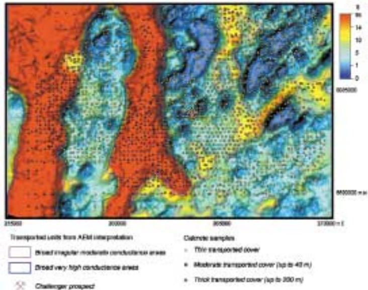
▲ **Figure 2.** Regolith conductance image for the Challenger area, overlain by calcrete sample locations classified according to the thickness of transported cover interpreted from AEM.
