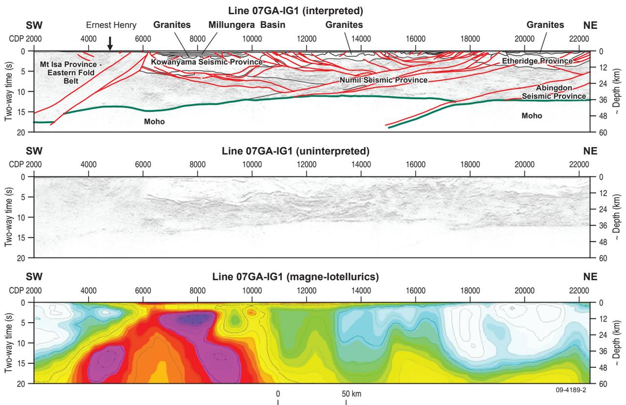
**Figure 2.** Images of traverse 07GA-IG1 showing (from top to bottom) interpreted seismic section, uninterpreted, migrated seismic section, and electrical resistivity from 2D inversions of magnetotelluric data.
