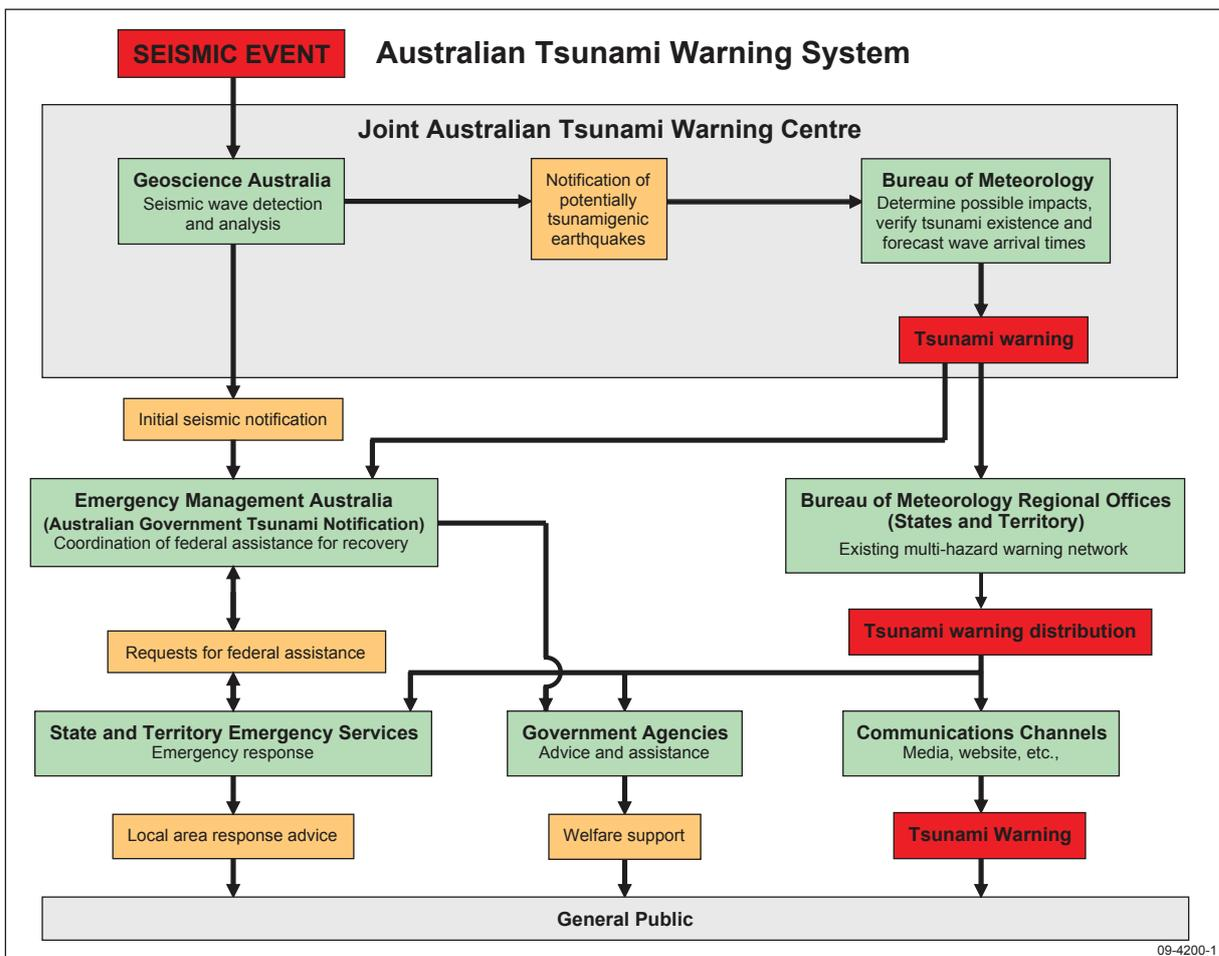
Figure 2. Flow chart outlining the roles of the contributors to the Joint Australian Tsunami Warning Centre operations.
