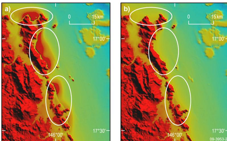
**Figure 3.** False-colour images showing the reduction to the interpolation artefacts between the continental shelf and land areas using the improved interpolation process. Comparison of the 2005 version of the grid (a) and the 2009 version (b) with variations highlighted by circled areas.
