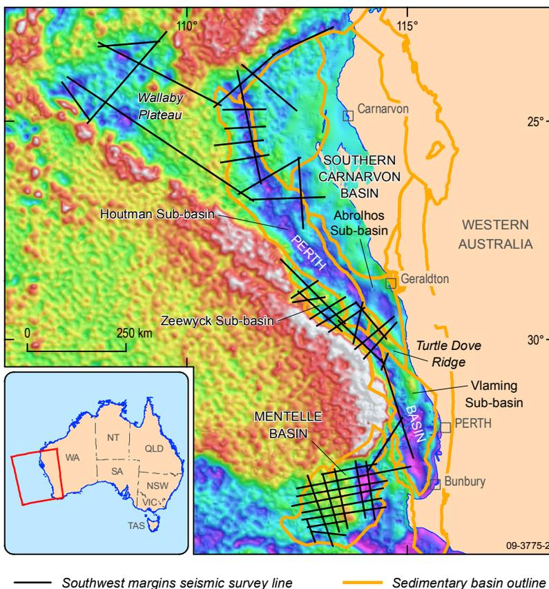
**Figure 1.** Seismic lines acquired during the Southwest Margin 2D seismic survey by the MV *Duke*. The background image is Bouguer-corrected satellite gravity data.
