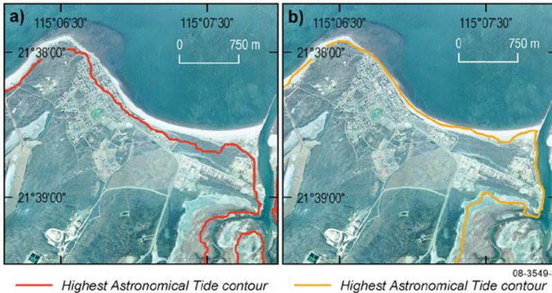
**Figure 3.** Data errors: accuracy in topography. Image shows highest astronomical tide contour for two data sets (a) 30 metre Digital Terrain Elevation Data Level 2 and (b) Landgate 20 metre Orthophoto Digital Elevation Model. Image courtesy of Landgate.
